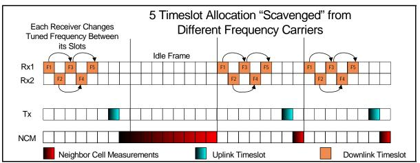
Through intelligent selection, a dual-carrier receiver architecture can support either dual-carrier reception or mobile-station receive diversity, depending on the operating environment.
