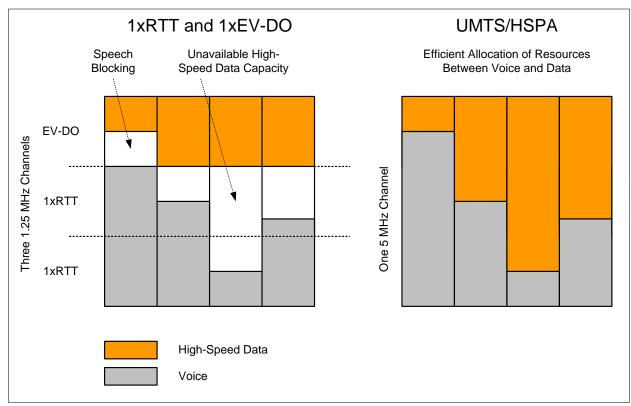
Figure 10: Radio Resource Management 1xRTT/1xEV-DO versus UMTS/HSPA
