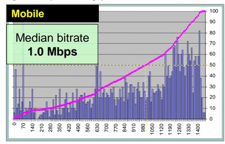
Figure 13: Uplink Throughput in a Commercial Network<sup>61</sup>
