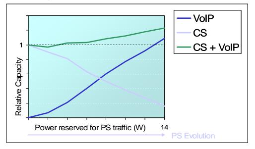
Figure 36: Ability for UMTS to Support Circuit and Packet Voice Users<sup>100</sup>
