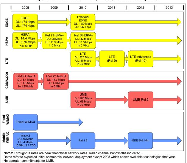
Figure 5: Evolution of TDMA, CDMA, and OFDMA Systems
