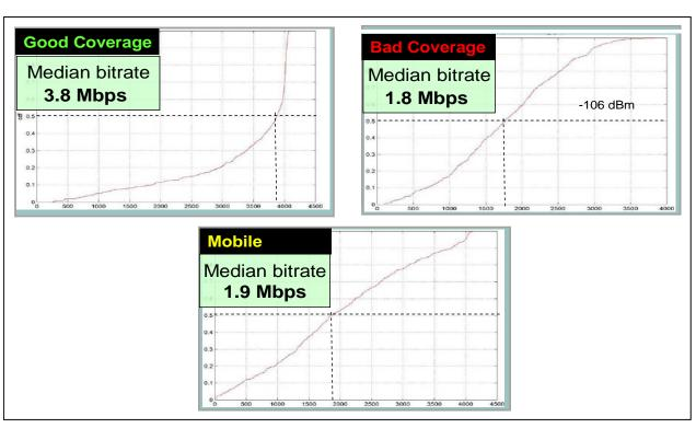
Figure 12: HSDPA Performance of a 7.2 Mbps Device in a Commercial Network<sup>59</sup>
