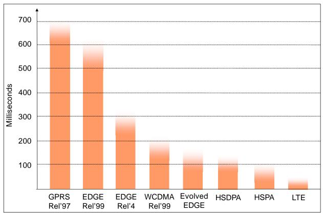
Figure 15: Latency of Different Technologies<sup>65</sup>
