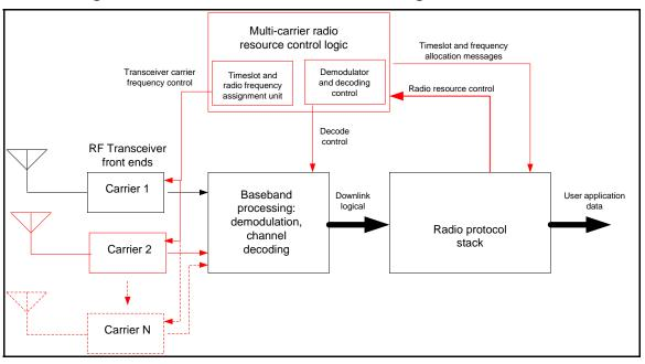
Figure 24: EDGE Multi-Carrier Receive Logic – Mobile Part<sup>86</sup>
