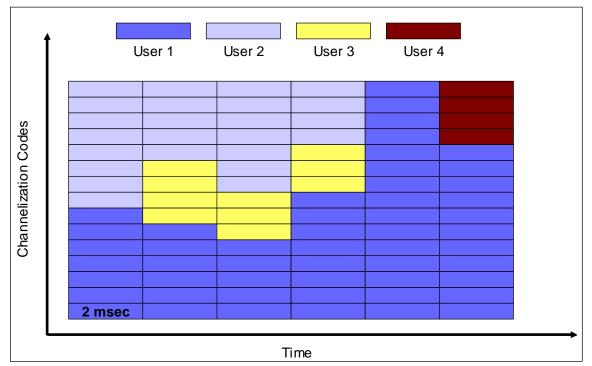
Figure 29: High Speed–Downlink Shared Channels (Example)
