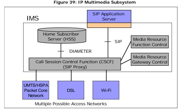
As shown in Figure 39, IMS operates just outside the packet core.
