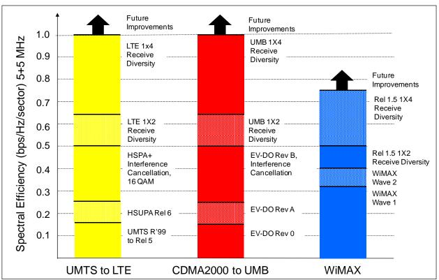
Figure 18: Comparison of Uplink Spectral Efficiency<sup>70</sup>
